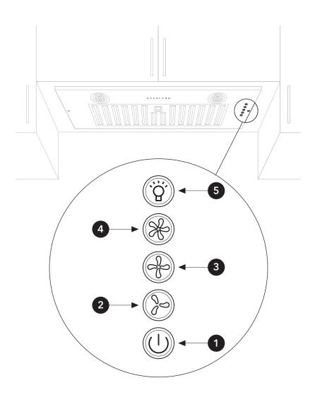
1- On/Off 2- Low Speed 3- Medium Speed 4- High Speed 5- Light
