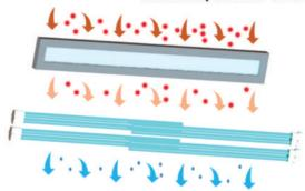
Photocatalytic Filter: a.k.a. Titanium Dioxide filter, changes the chemical makeup of harmful pollutants into harmless byproducts of water and oxygen.
