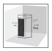
Do not obstruct the air intake or the clean air outlet. To ensure proper air circulation, leave at least 10" space between the back air intake and the wall or the furniture.
