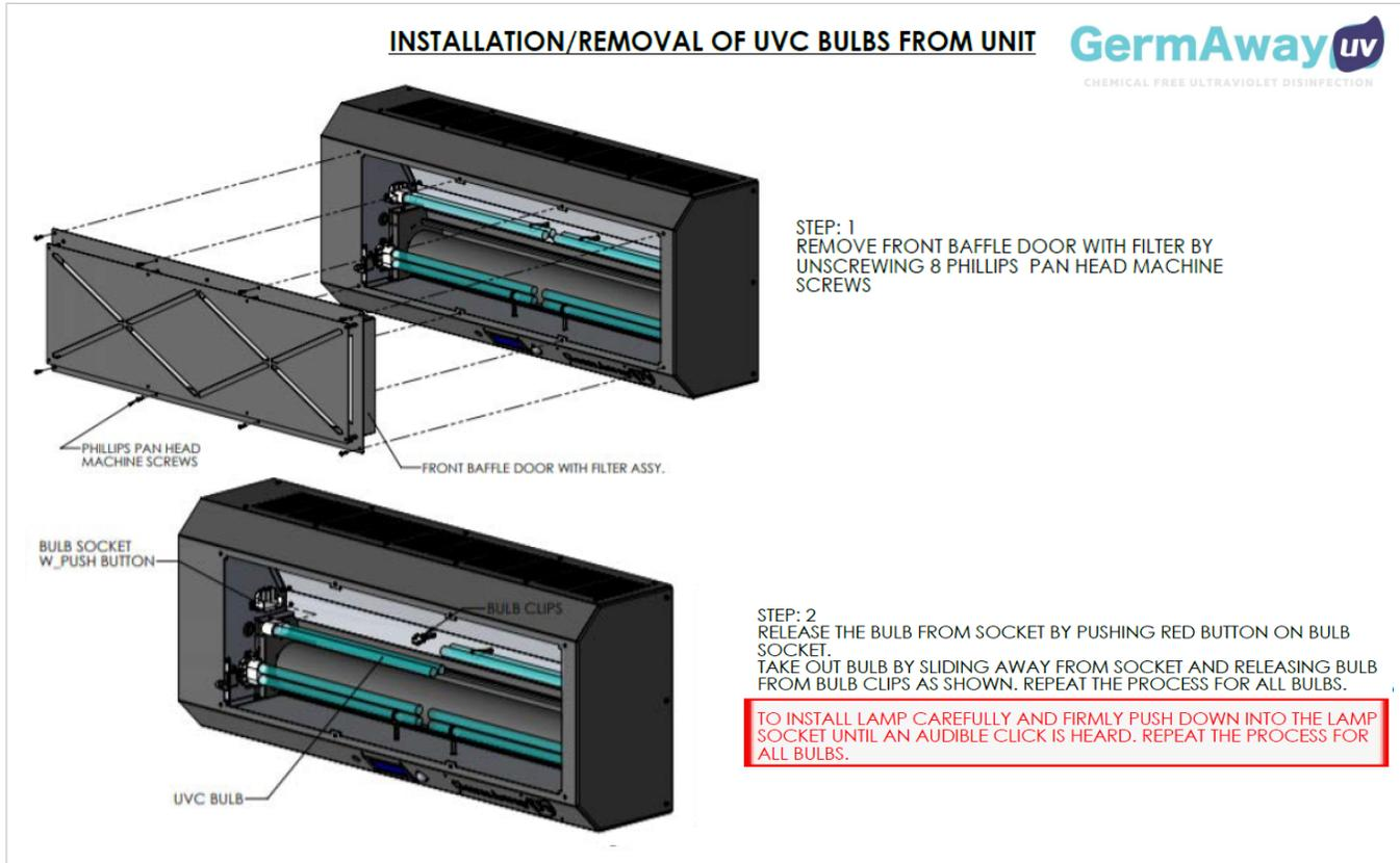
**Step 1:** Remove Front Door with Filter by unscrewing 8 captive screws.
